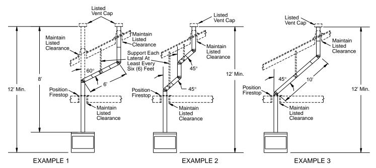
Figure 10 - Typical B-Vent Configuration
